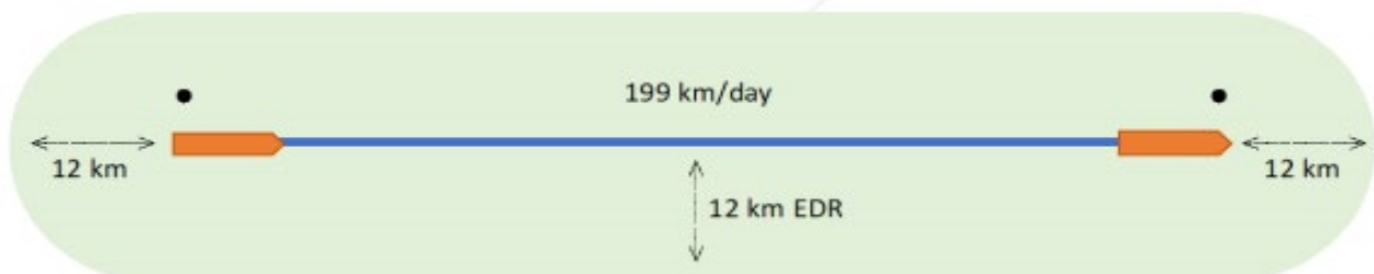
Figure 7.21: Maximum worst-case theoretical area of impact over a single day from a seismic survey travelling 199 km/day at 4.5 knots using 12 km EDR (BEIS, 2020).
