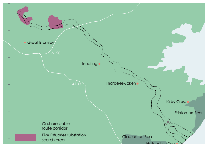
Figure 3: Overview of the Project's underground cable route corridor and search areas for the proposed onshore substation
